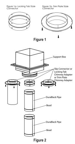
certain amount of spacing at the joints, which may in some cases permit creosote leakage. If the ceiling is higher than 8 feet, obtain Pipe Sections from your dealer to accommodate the additional height. See dealer for available pipe section lengths.
